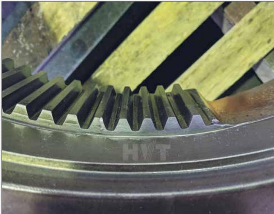
Weld repair of cracked splines on a cast iron CAT 793 extended life rear brake housing, proving a challenging solution to maintenance gaps in today's industry.
