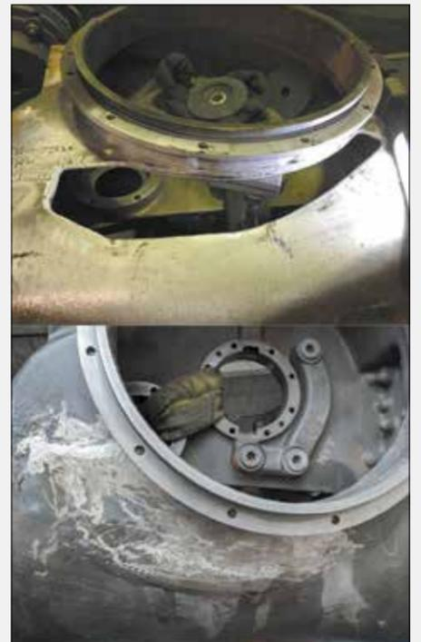
When there is no new, used will most-certainly do. A remarkable recovery of a badly damaged cast iron converter case using high-temperature forge welding techniques.
